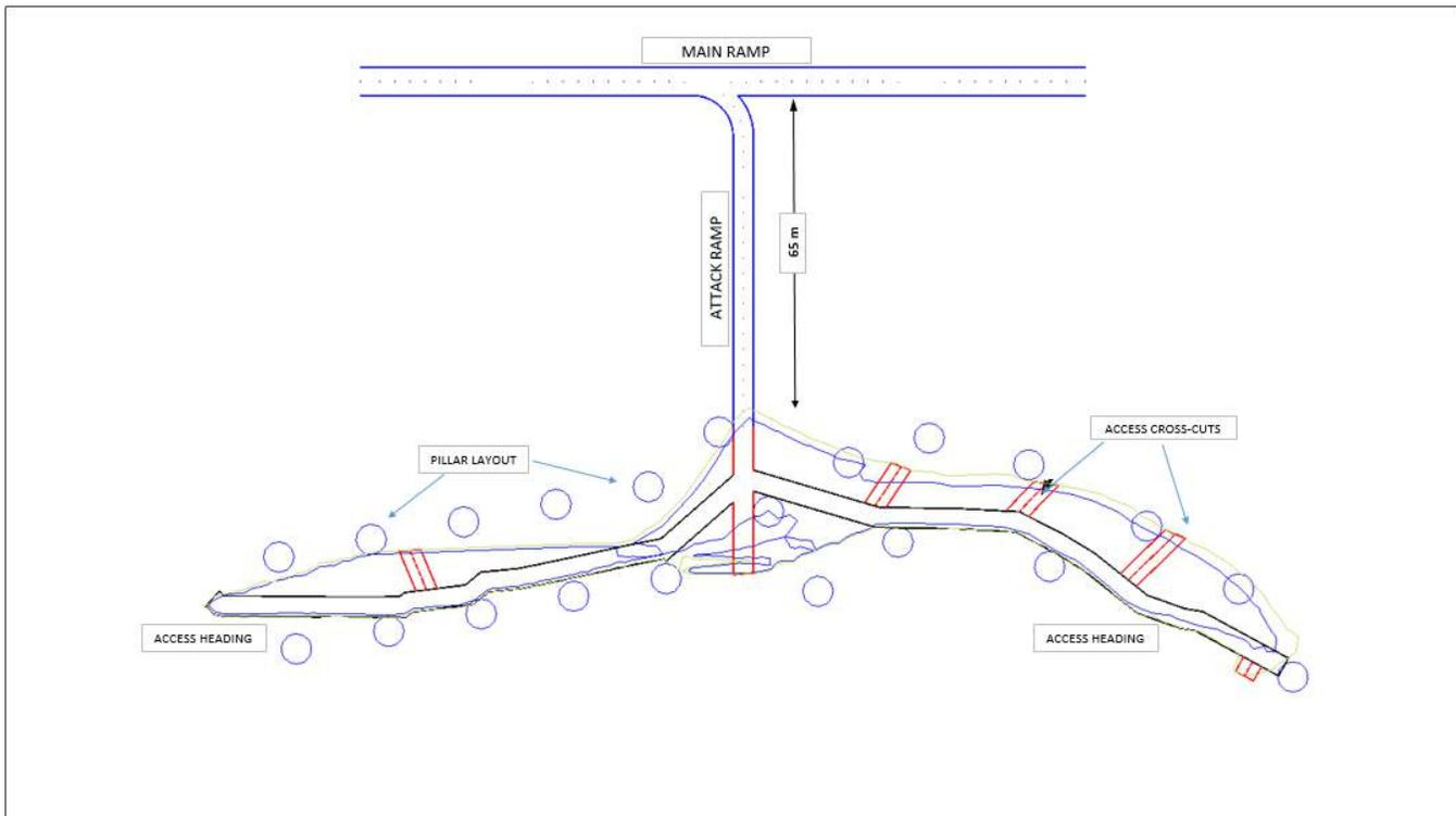
**Figure 16.4 Typical Mining Panels with Attack Ramp Access**
