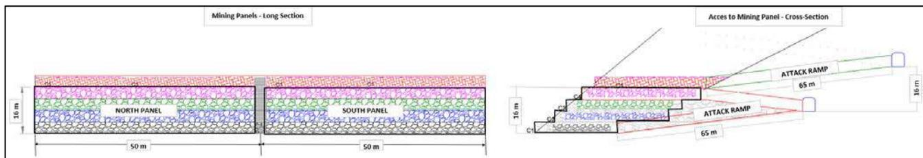
Once each lift is mined out it will be back filled with waste material from the various access development headings and, if necessary, with material hauled from the La Estrella quarry, located 3km from the North Portal.
