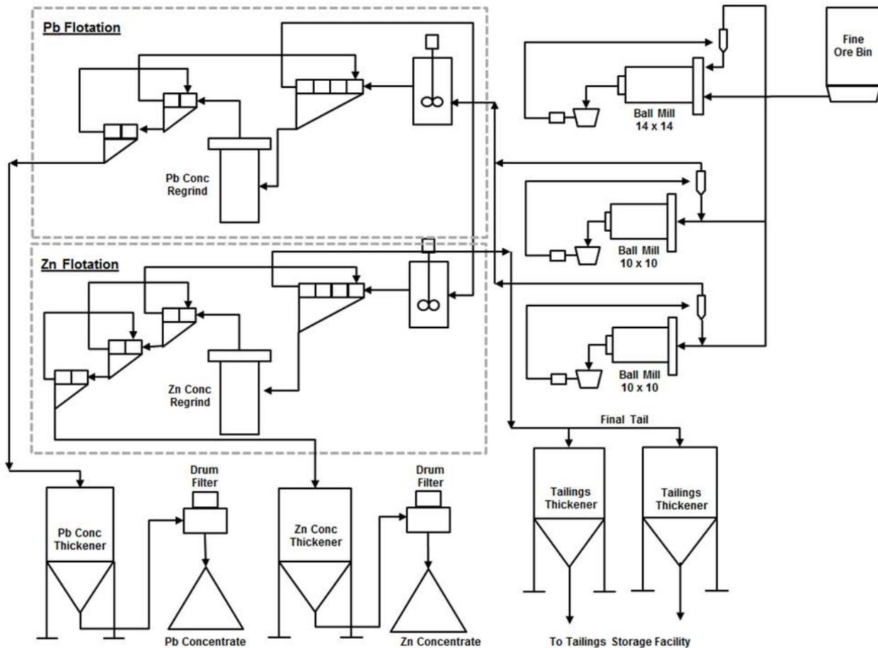
To process the San Rafael sulfide ore at 1,800 tonnes per day and a  $P_{80}$  of 106 $\mu$ m, additional grinding capacity is required and will be in the form of a 3.4 meter diameter, 4.3 meter long 1,119 kW ball mill. This mill will serve as the primary grinding mill and will discharge to the existing two ball mills currently serving as primary mills. The new grinding mill and much of the infrastructure exists at the plant site today, but remains to be installed and commissioned.
